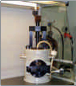
Gene gun used for introducing new genes into sugarcane cells.
